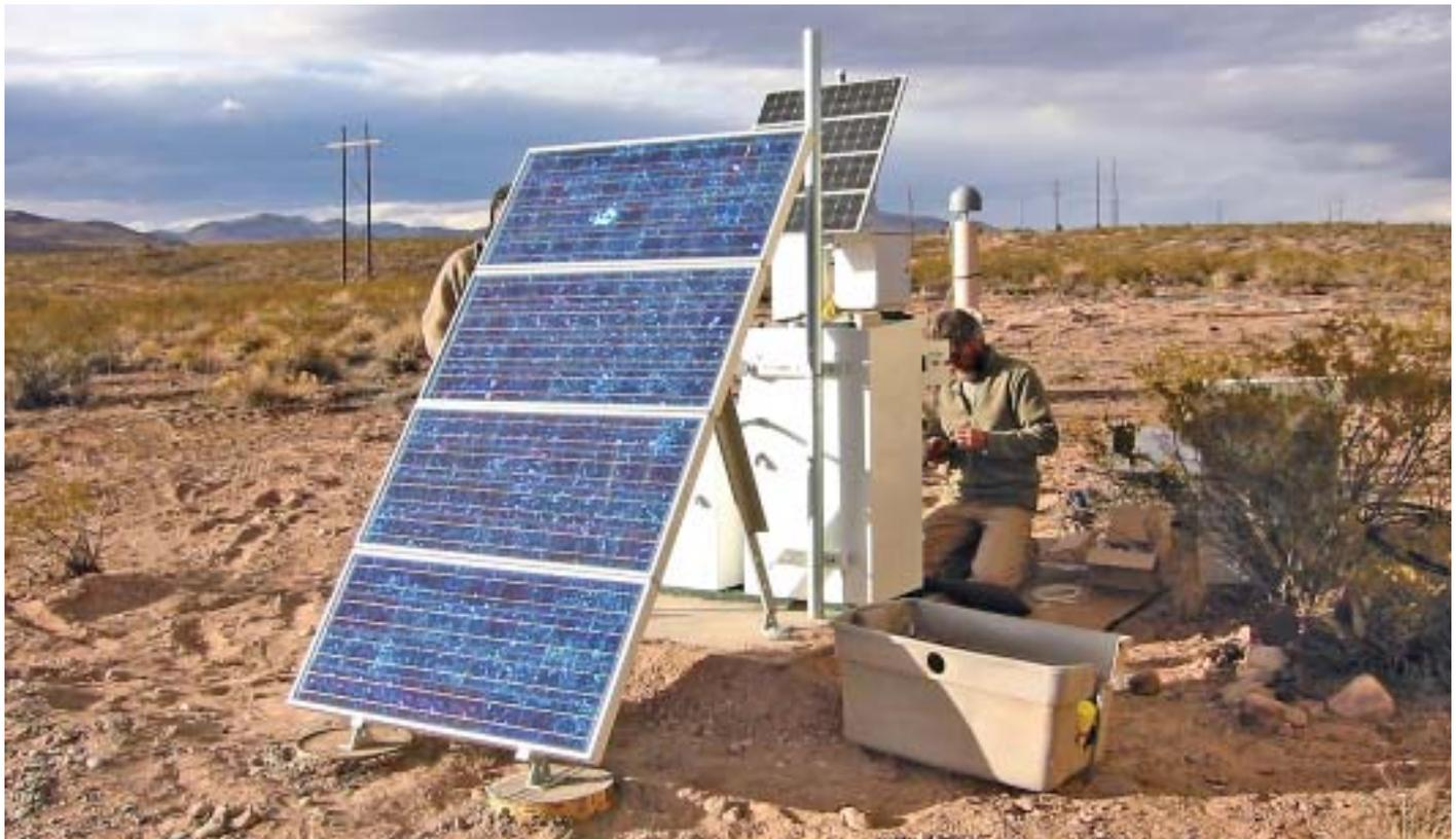
**Figure 1:** Deployment of a seismic station in the “Bigfoot” array, an integral part of the USArray Transportable Seismic Network. Photo courtesy of EarthScope.
