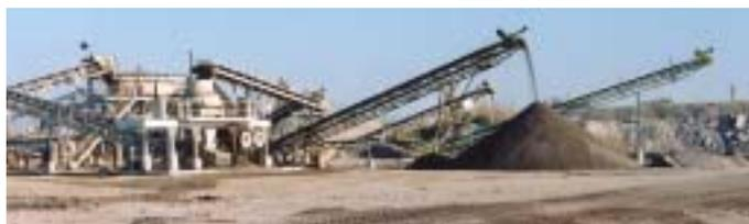
**Figure 3** Sand and gravel being sorted by particle size.
