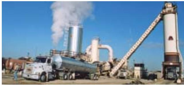
**Figure 4** (Left) Sand and gravel being mixed with cement to produce concrete. **Figure 5** (Above) Sand and gravel being mixed with hot oil to produce asphalt.
