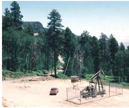
Figure 3. Pumping unit on producing oil well. Note car for scale.
