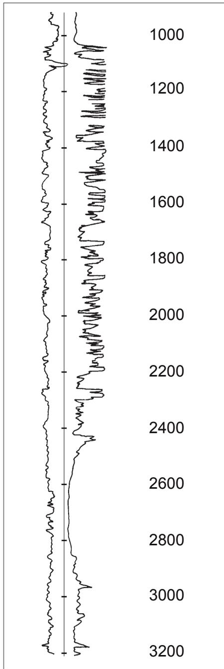
Figure 2. Segment of typical well log. Curve deflections indicate rock properties that can be correlated from well to well. Numbers represent depth in feet below surface .
