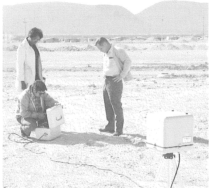
**Figure 2 (above).** Gamma radiation being measured by Ralph B. Ochoa (kneeling, left) and Mattie Coleman (standing, left), both of the Arizona Atomic Energy Commission. Richard T. Moore, Arizona Bureau of Mines (right), observes. Photo taken by John S. Vuich, Arizona Bureau of Mines, February 25, 1976.
