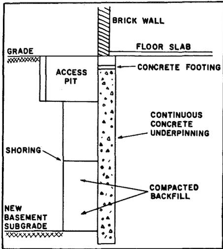
Figure 7. A cross section of the continuous underpinning method of stabilizing existing foundations.
