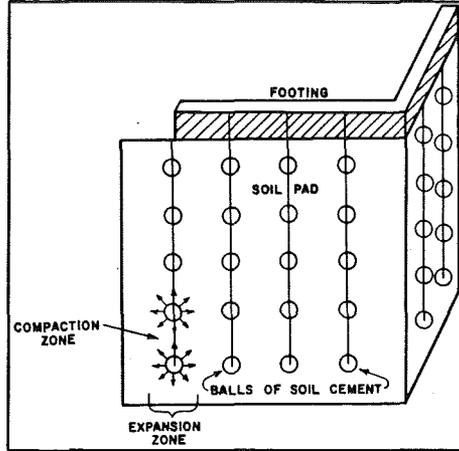
Figure 8. A demonstration of the soil-cement injection method of stabilizing damaged foundations.
